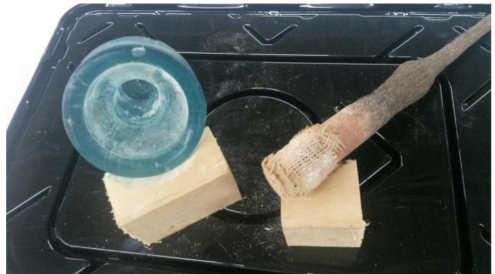
Here is a photo of Roy Hale's display at the February swap meet, which featured an unembossed CD 731 threadless insulator that came with it's original pin. The photo below shows a close-up of the pin, with the remarkably preserved burlap that helped hold it to the insulator. Not sure what the white substance on the burlap is.
